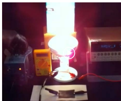
Figure: Demonstration of PEDOT-PSS treated synthetic leather (rectangular fabric connected to alligator clips) carrying 2 Amps at AC 120V to light a 240 Watt heatlamp.
